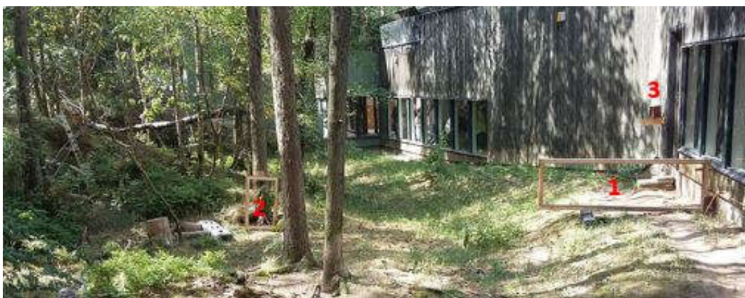
Figure 4: Automated monitoring. 1 : HDX PIT tag “pacing” antenna, 2 : Scent station with HDX PIT tag “scent” antenna, 3 : Reconyx Hyperfire wildlife camera, 4 : BLE tag logging smartphone.
