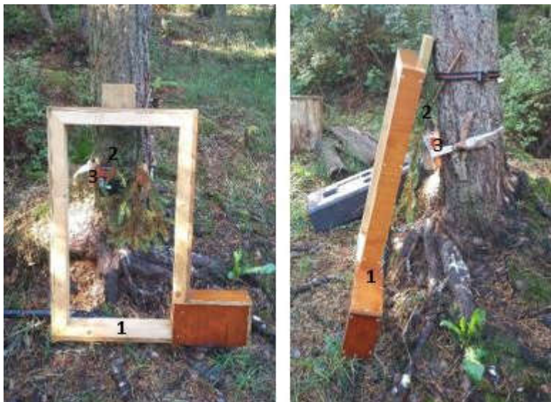
Figure 3: Scent station. 1 : HDX PIT tag antenna. 2 : Spruce branch, 3 : BLE tag logging smartphone inside a waterproof plastic box
