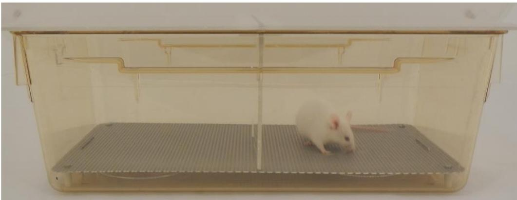
**Figure 1:** Side view of the test arena with dividing wall in the middle, perforated floor on the bottom, and plexiglas lid on top.
