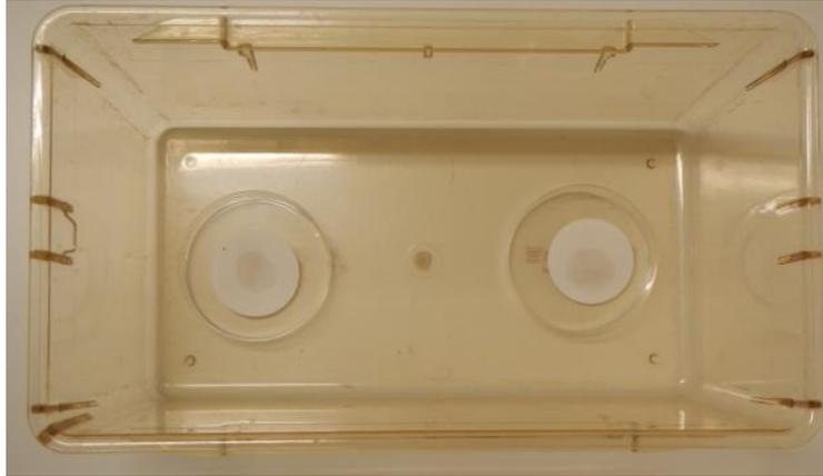
**Figure 2:** Top view of the test arena with the impregnated petri dishes in position and the perforated floor removed.
