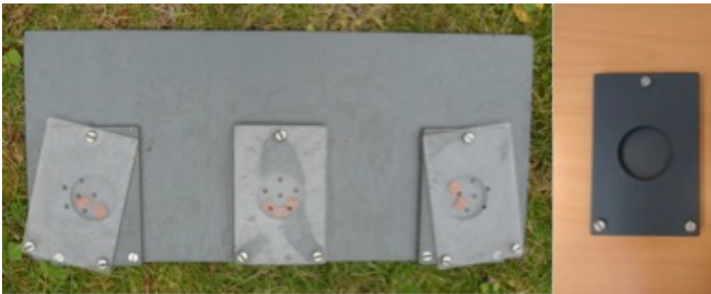
Figure 1 A: The problem-solving test setup (54.8 x 24.8 cm) with treats, side slabs slightly open. B: The motivation test plate (15 x 9.8 cm).
