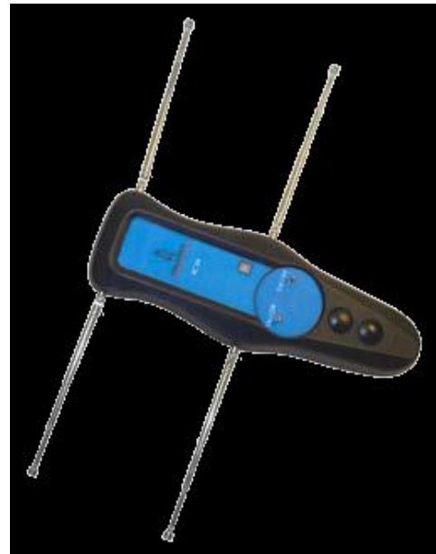
Figure 2a: The Tellus GPS-collar with UHF (Ultra High Frequency) data transfer. Figure 2b: The RCD-04 receiver used to upload data from the collar.
