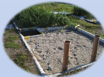
Two of the pilot-scale VF CWs; one planted and one unplanted.
