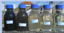
Wastewater samples collected from inlet (0 cm depth), 3 internal sampling points (10, 20 and 40 cm depth) and outlet (80 cm depth) in a sand VF CW. Note the color difference from inlet to outlet.
