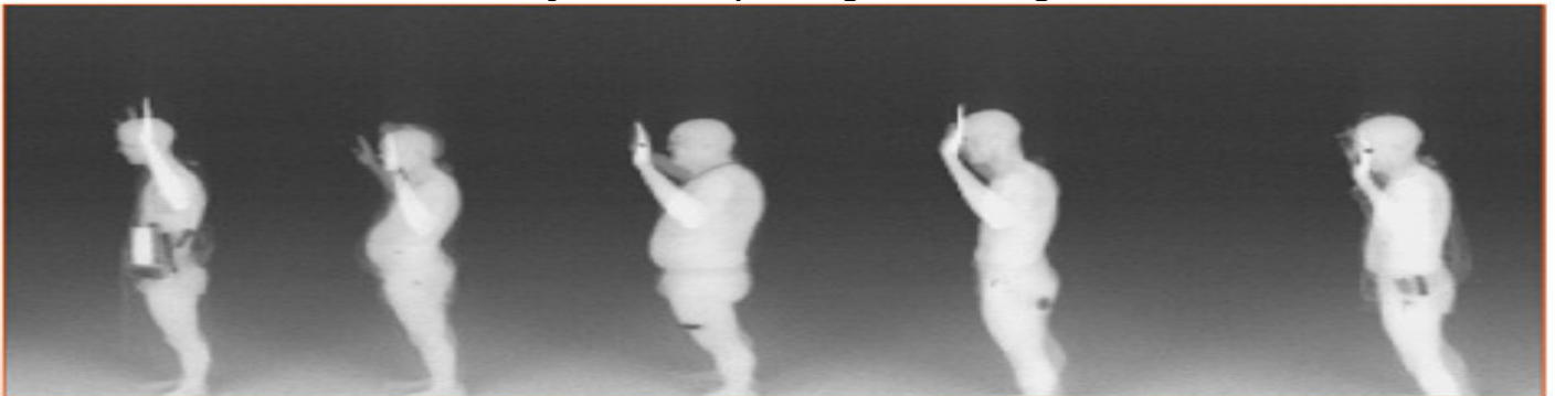
Standoff X-ray detection showing hidden explosives and other items on personnel. Images were taken from a van moving at 0.3 to 6 miles per hour using X-ray backscattering in "drive-by" mode. The mock suicide vest contained simulated C4 explosives and pipe bombs. Both the explosives and the pipe bombs are easy to see and are distinguishable from normal objects under clothing.
