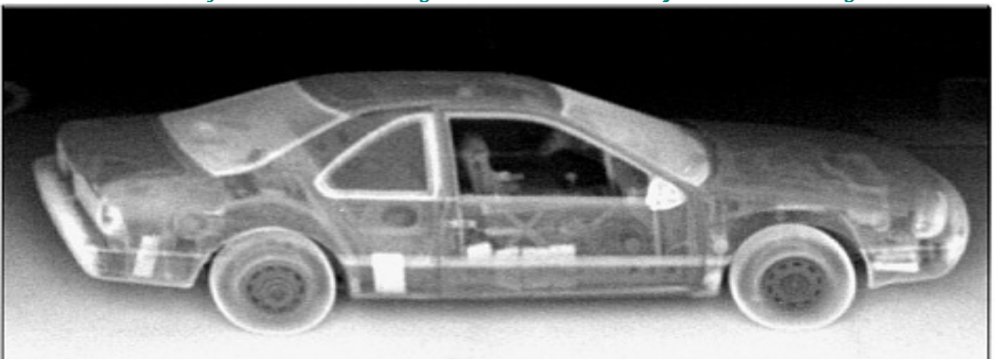
X-ray image of a car containing C4 explosive packages (just in front of the front wheel, to the rear of the door, in the roof just above the door, and in the back fender), drugs (in the door), and a 150 pound ANFO (ammonium nitrate-fuel oil) bomb with a grenade detonator (in the trunk).
